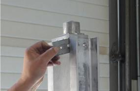
Remove the four (4) button head cap screws (3/16" Allen key) holding the outer frame to the screw assembly ballnut bracket.
