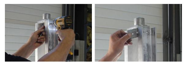
Remove the four (4) button head cap screws (3/16" Allen key) holding the outer frame to the screw assembly ballnut bracket.
